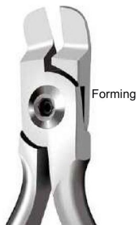
Tweed B-12-4611 T/C 11.5 cm/ 4½" Rectangular Arch Pliers, Tweed Style Forming plier for square or rectangular wires. The blades are designed to be parallel at .020" ( 0.51 mm ) opening. The working edges are carefully diamond-honed to prevent wire scoring.
